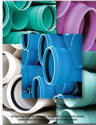
This document covers PVC pressure pipe for potable water, reclaimed water, and sewer forcemain systems; and PVC non-pressure pipe for storm sewer and sanitary sewer systems. All pipes are made in lengths that are assembled at the job site. Each length has a belled end with an elastomeric gasket such that each pipe length's spigot end fits inside the belled end of the next pipe length.
